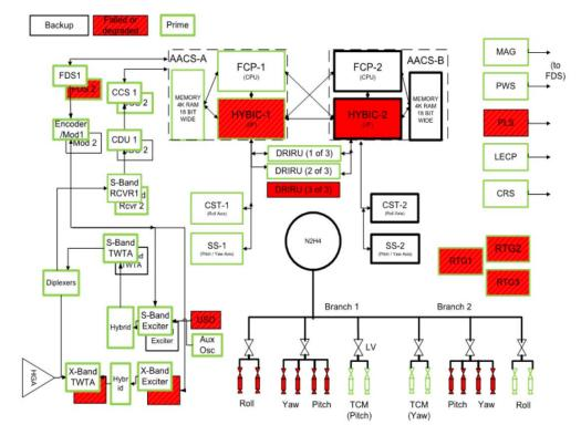
Figure 2. The system architecture for Voyager 2. Note that most of the actuators are non-operational.
