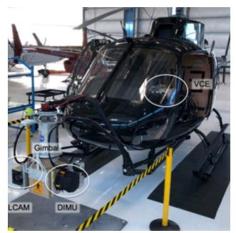
Figure 1. The helicopter test rig. LCAM, DIMU, and VCE corresponds to LVS Camera, Descent Inertial Measurement Unit, and Vision Compute Element.
